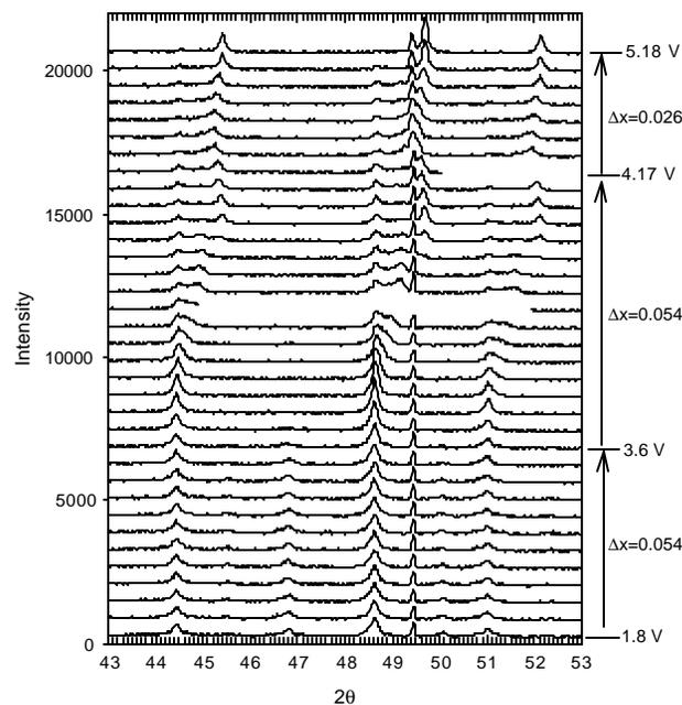
**Figure 37.** XRD patterns for  $\text{Li}_{1.1}\text{Mn}_2\text{O}_4$  during charge after a discharge to 1.8 V. The right ordinate indicates voltages at various stages of charge as well as the value of  $\Delta x$  for each scan.
