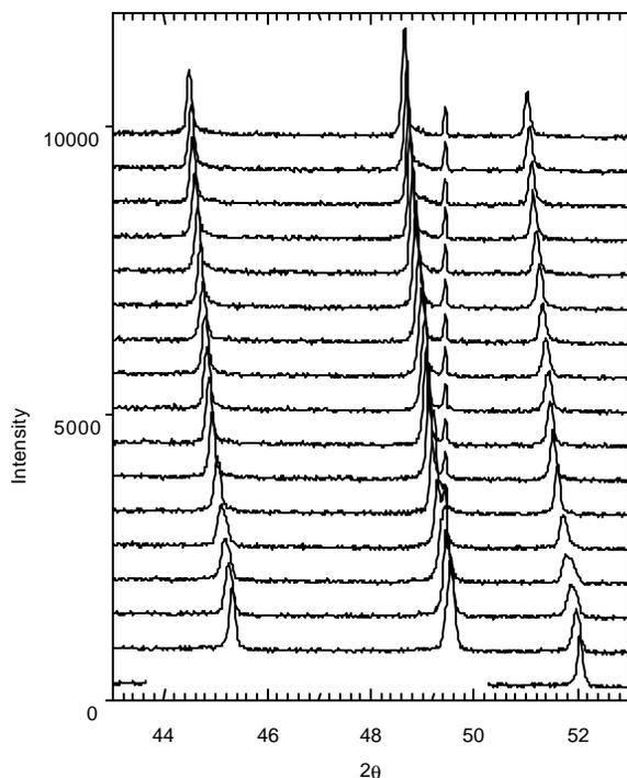
**Figure 36.** XRD patterns for  $\text{Li}_{1.1}\text{Mn}_2\text{O}_4$  for the first discharge from 4.5 to 3.5 V at C/8 rate. The change in  $\text{Li}_x$  content during each scan,  $\Delta x=0.065$ . Bottom scan beginning of discharge, top scan end of discharge.
