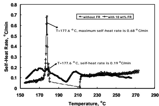
**Figure 10.** Thermal behavior of 1 M LiPF<sub>6</sub> with EC-DMC containing 0.0 and 10.0 wt% of the HMTAP flame-retardant additive using ARC.
