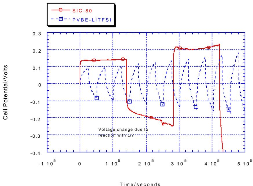
**Figure 25.** Cycling behavior of Li/Li symmetrical cells at 85°C. Both cells are cycled galvanostatically at 0.05mA/cm<sup>2</sup>. SIC-80 is a polyelectrolyte with a glass transition temperature of -51°C and a conductivity of 10<sup>-5</sup> S/cm at 85°C. The PVBE polymer is a cross-linked polyvinylbenzyl ether with a side chain length of 12 EO units.
