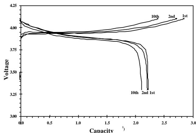
Figure 12. Charge/discharge cycles for a Li/LiCoO<sub>2</sub> cell using the 1:1 EC/TFEA- LiC(SO<sub>2</sub>CF<sub>3</sub>)<sub>3</sub> (1M) electrolyte.  $I_d = I_c = 0.25 \text{ mA/cm}^2$
