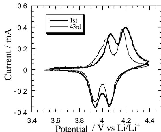
Figure 33. Cyclic voltammograms of a thin-film LiMn<sub>2</sub>O<sub>4</sub> electrode in 1 M LiPF<sub>6</sub>-EC-DMC electrolyte, recorded at 1 mV/s.
