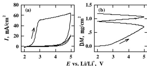
**Figure 9.** (a) cyclic voltammogram and (b) simultaneously acquired mass change diagram for an Al electrode polished with a SiC cloth during the first two cyclic scans in 1 M  $\text{LiPF}_6/\text{PC}$ .
