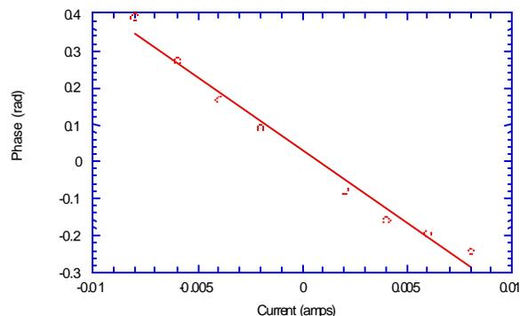
**Figure 32.** Phase shift of  $^{19}\text{F}$  signal vs. applied current for a sample of 0.292 M Li methide in PEGdm and 5% R805 fumed silica. The slope is proportional to the anion transference number. The negative slope is a result of the fact that the anions migrate in the opposite direction ( $-Z$ ) of the cations.
