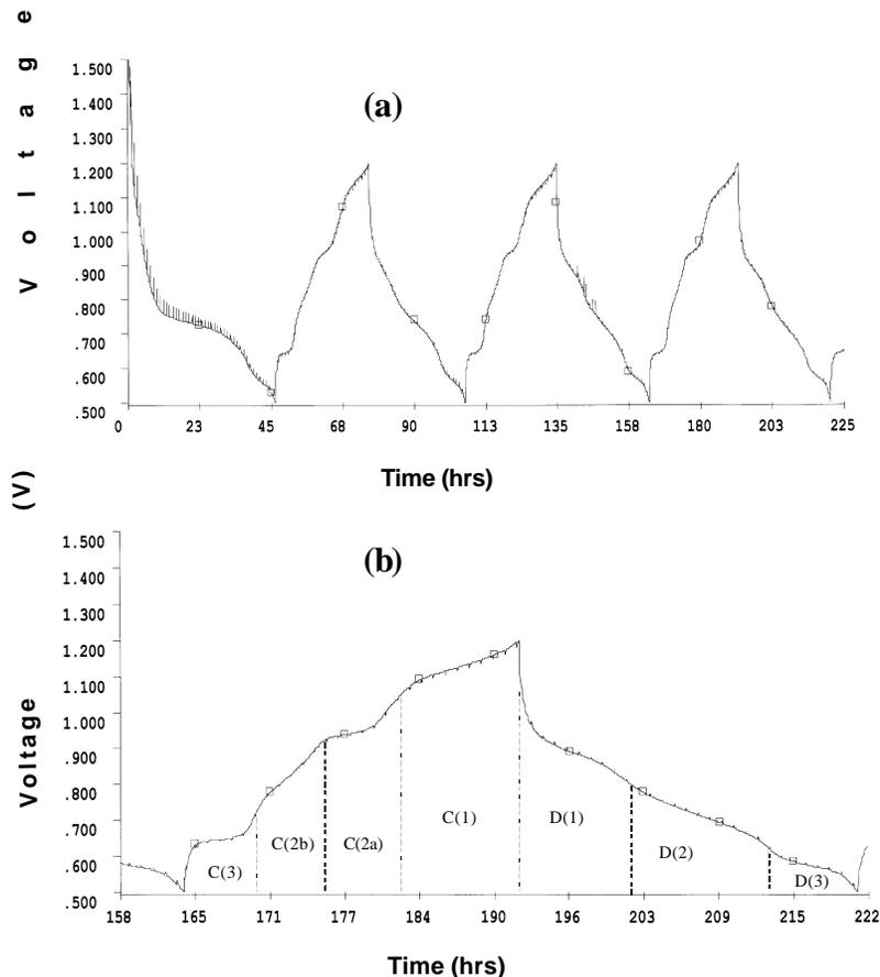
**Figure 13.** Electrochemical characteristics of a Li/InSb cell: (a) the voltage profile (first 3 cycles) between 1.2 and 0.5 V, and (b) an enlarged representation of the 3rd charge and discharge cycles.
