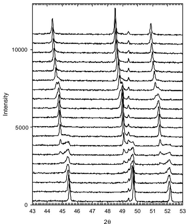
**Figure 35.** XRD patterns for  $\text{Li}_{1.0}\text{Mn}_2\text{O}_4$  for the first discharge from 4.5 to 3.5 V at C/8 rate. The change in  $\text{Li}_x$  content during each scan,  $\Delta x=0.053$ . Bottom scan beginning of discharge, top scan end of discharge.
