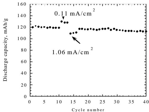
**Figure 23.** Cycling data for cell A8, discharged between 4.0 and 2.3V at 0.53 mA/cm<sup>2</sup> (~C rate), except where otherwise noted. Forty cycles at different rates, voltage limits are not shown.
