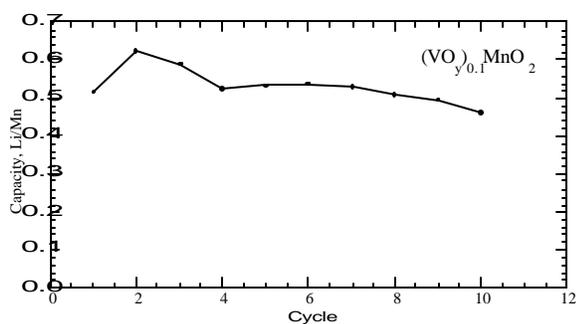
Figure 18. Capacity on cycling of  $(VO_y)_{0.1}MnO_2$ .
