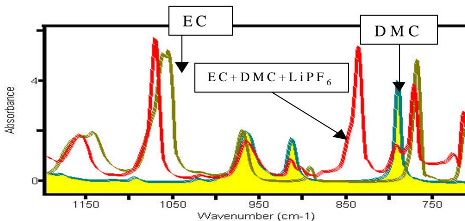
**Figure 3.** Raman spectra of ethylene carbonate, dimethyl carbonate, and electrolyte (EC+DMC+1M $\text{LiPF}_6$ ). The results indicate preferential solvation of the Li ion.
