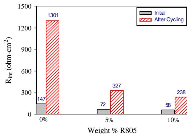
**Figure 28.** Effect of fumed silica content on interfacial resistance before and after cell cycling. Samples are PEG-DME, Li imide (Li:O=1:20), and R805 fumed silica in a Li/CPE/Li button-cell. Interfacial resistance measured before and after cycling via AC impedance spectroscopy; 584 cycles were applied to the 5 and 10% R805 samples, but only 327 cycles were applied to the 0% sample due to the equipment limitations (impedance of cell became too large).
