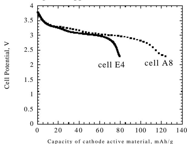
**Figure 22.** Discharges at 0.53 mA/cm<sup>2</sup> (~C rate) of two  $\text{Li}_x\text{MnO}_2/\text{EC-DMC}$ , 1M  $\text{LiPF}_6/\text{Li}$  cells at room temperature. The  $\text{Li}_x\text{MnO}_2$  sample used in cell A8 was attritor-milled for four hours.
