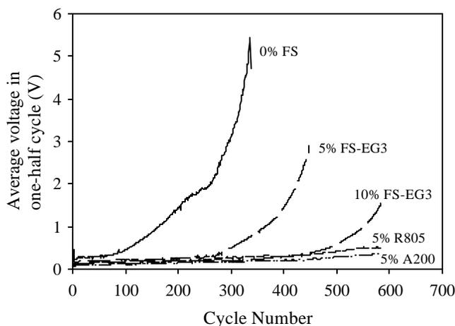
**Figure 27.** Effect of fumed silica surface groups on interfacial stability at 1 mA/cm<sup>2</sup>. Samples are PEG-DME, Li imide (Li:O=1:20), and fumed silica: OH terminated (A200), oligomer ethylene oxide terminated (FS-EG3), and octyl terminated (R805). Samples are assembled as at Li/CPE/Li button-cell with moisture content < 40 ppm.
