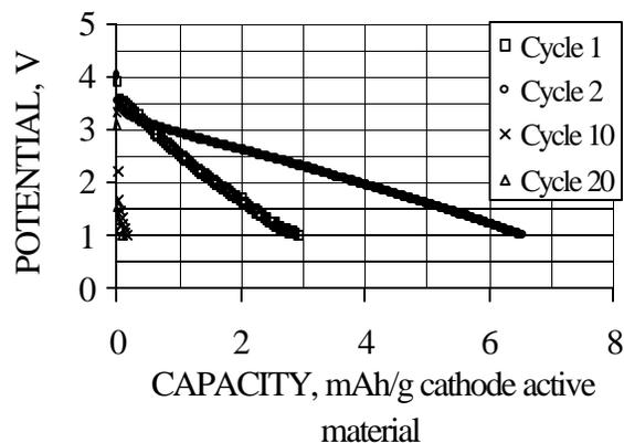
**Figure 29.** Discharge of Li/(PVICOX)/ LiMn<sub>2</sub>O<sub>4</sub>;C; MEEP-lithium triflate cell at 25°C. Discharge current 8 mA/cm<sup>2</sup>.
