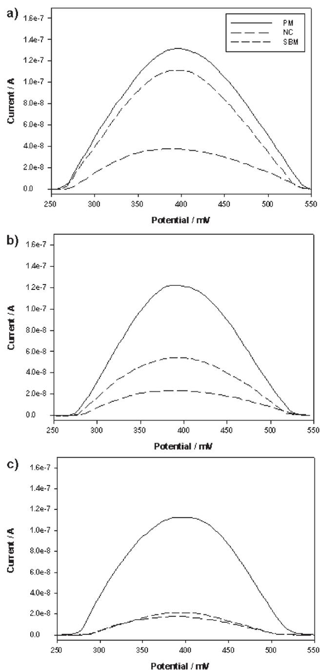
Fig. 4. The baseline-corrected DPV response of electrodes with enzymatic reaction by S1 nuclease at a) room temperature, b) 37 °C, and c) 50 °C after three different target hybridization on the gold electrode modified with Fc ss-DNA probe. The pulse amplitude was 0.05 V and the scan rate was 0.02 V/s.
