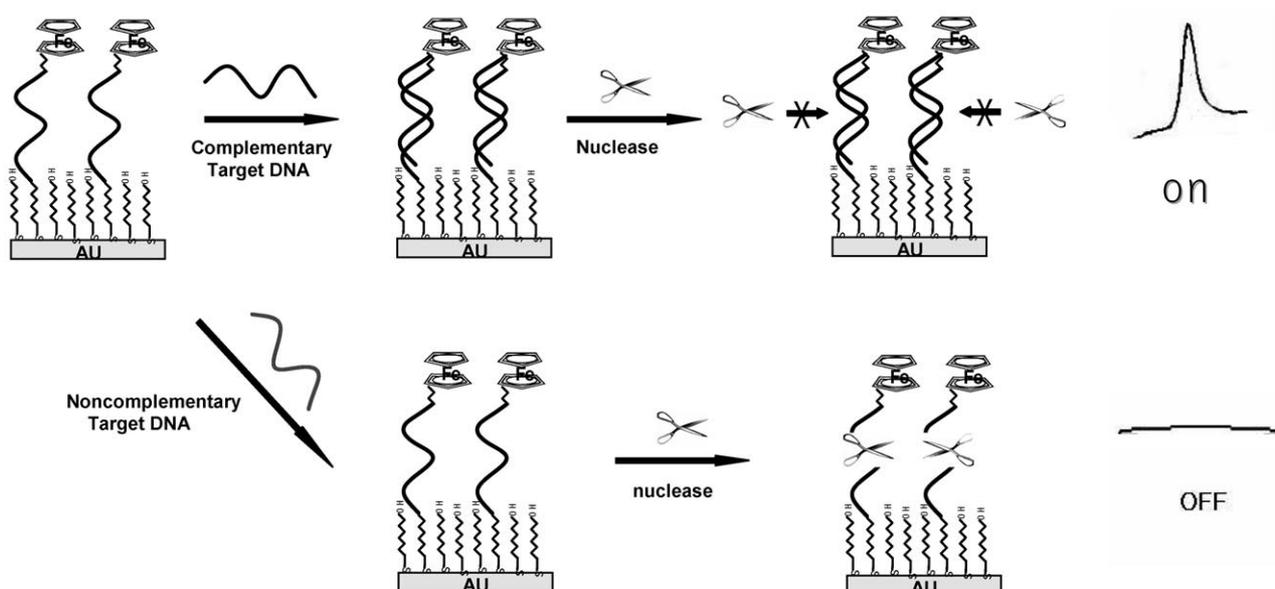
Fig. 1. Schematic illustration of DNA detection using S1 nuclease.
