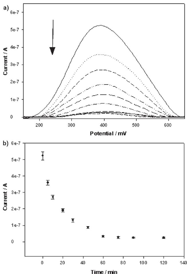
Fig. 3. The baseline-corrected DPV of Fc ss-DNA modified electrode with enzymatic reaction by S1 nuclease at different reaction time (0–120 min) (error bar is three times) (a). Plot of peak currents with the increasing time (b). The pulse amplitude was 0.05 V and the scan rate was 0.02 V/s.
