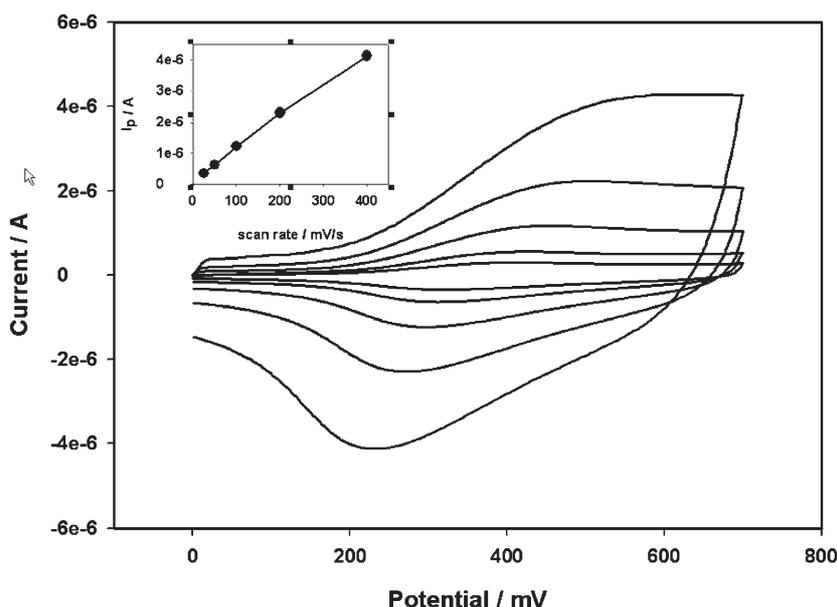
Fig. 2. Cyclic voltammogram of Fc ss-DNA modified electrode dependent on a scan rate from 25 to 400 mV/s in 0.1 M HClO<sub>4</sub>. Inset: Plot of anodic peak currents to potential sweep rates.
