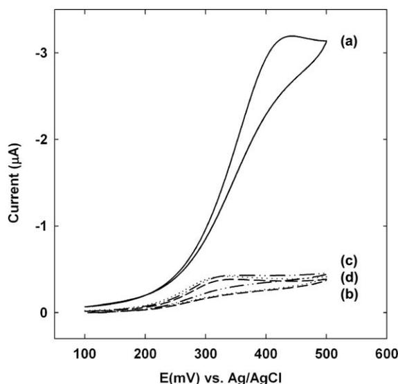
**Fig. 6** Cyclic voltammograms of a sandwich-type electrochemical immunosensor for mouse IgG at (a)  $1 \text{ ng mL}^{-1}$  mouse IgG, (b)  $0 \text{ g mL}^{-1}$  mouse IgG, (c)  $10 \mu\text{g mL}^{-1}$  PSA, and (d)  $10 \mu\text{g mL}^{-1}$  thrombin. All cyclic voltammograms were obtained after incubating for 10 min in EB containing 1 mM APP and 5 mM NADH at a scan rate of  $10 \text{ mV s}^{-1}$ .
