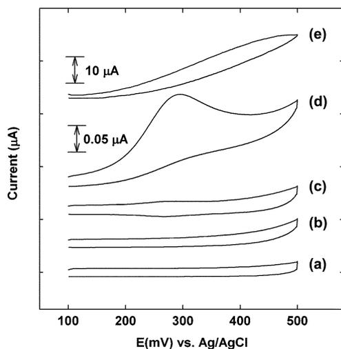
**Fig. 1** Cyclic voltammograms of SAM-modified Au electrodes in (a) EB and (b) EB containing 5 mM NADH, and cyclic voltammograms of SAM- and 0.5% Fc-D-modified Au electrodes in (c) EB and (d) EB containing 5 mM NADH, and bare Au electrodes in (e) EB containing 5 mM NADH at a scan rate of 10 mV s<sup>-1</sup>. The scale bars: 0.05 µA for (a)–(d), and 10 µA for (e).
