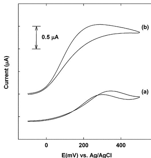
**Fig. 5** Cyclic voltammograms of 5 mM hydrazine in EB at (a) the SAM-modified and (b) the 0.5% Fc-D-modified Au electrodes at a scan rate of  $10 \text{ mV s}^{-1}$ .
