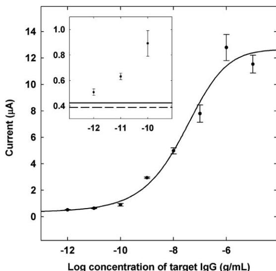
**Fig. 4** Calibration plot obtained from Fig. 3. The currents at 0.3 V are taken. The dashed line represents the mean of the current obtained in  $0 \text{ g mL}^{-1}$  mouse IgG. The solid line corresponds to the mean current at the zero concentration plus three times the standard deviation (SD).
