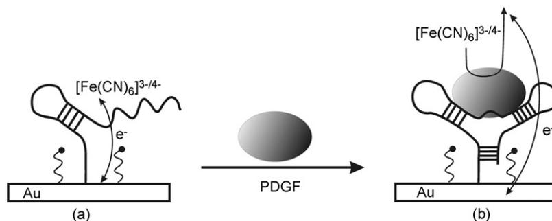
**Fig. 1 – Label-free electrochemical sensing of PDGF protein using PDGF binding aptamer self-assembled monolayers (SAMs) on a gold electrode and electrochemical transduction (a) before and (b) after target protein recognition.**
