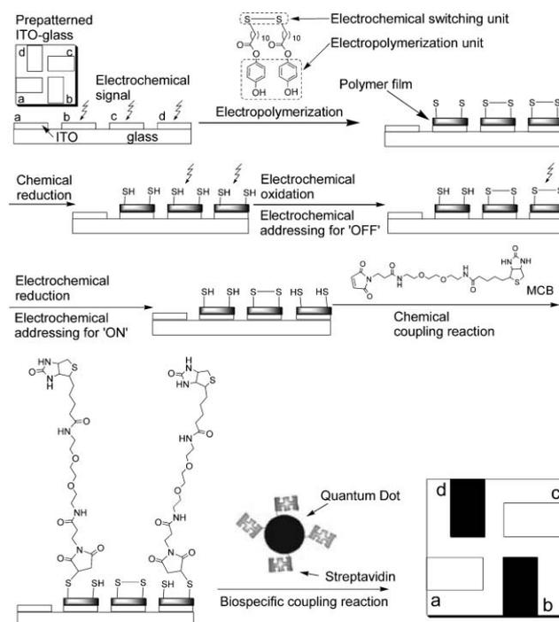
**Fig. 1** The chemical structure of HMDS employed in this paper and a proposed scheme for protein patterning by step-by-step modification of the ITO surface by chemical and electrochemical treatments.
