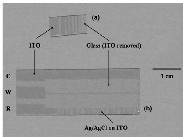
Fig. 1. Photograph of patterned ITO films: (a) lines with various widths; (b) an integrated ITO sensor consisting of a  $100 \mu\text{m}$  width band microelectrode, Ag|AgCl reference electrode and ITO counter electrode.
