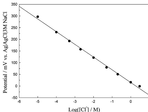
Fig. 2. Potential change of the fabricated Ag|AgCl reference electrode with varying concentrations of  $\text{Cl}^-$ .
