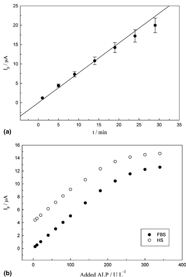
Fig. 5. Quantitative analysis of ALP activity: (a) peak currents proportional to exposure time to sample FBS containing 80 U/L ALP and (b) result of standard addition of ALP.
