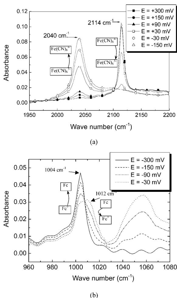
Fig. 8. a) In situ monitoring of spectroelectrochemical phenomena in 2 mM  $\text{Fe}(\text{CN})_6^{3-}$  solution with the potential of working electrode changing from 300 mV to  $-150$  mV. b) In situ FTIR spectra of 2 mM ferrocene in dichloromethane solution with varying working electrode potential.
