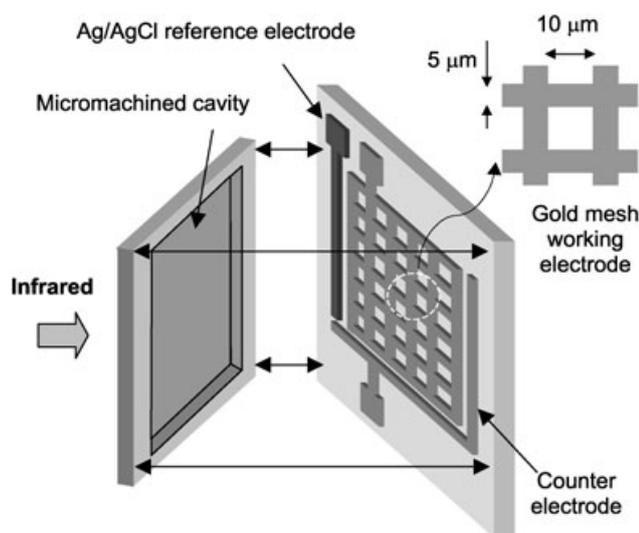
Fig. 1. Proposed structure of micromachined IR thin-layer cell.
