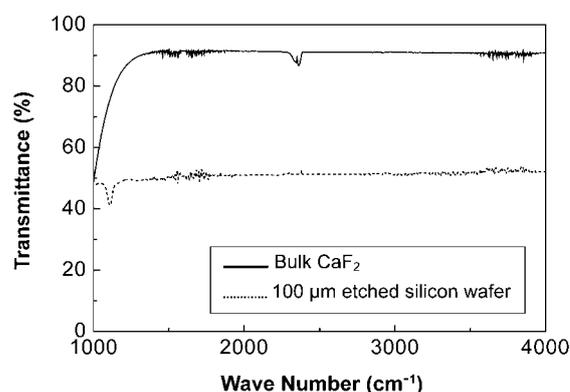
Fig. 2. FTIR transmittance of bulk CaF<sub>2</sub> plates compared with that of a double-side polished silicon wafer with a 100  $\mu\text{m}$ -etched cavity.
