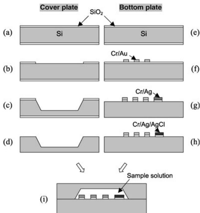
Fig. 3. Fabrication process of cover and bottom plates composing thin-layer cell and schematic view for thin-layer formation.
