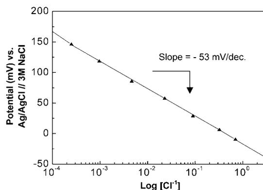
Fig. 5. Measured potential difference between the fabricated Ag/AgCl electrode and a commercial Ag/AgCl (dipped in 3 M NaCl solution) reference electrode as a function of various  $\text{Cl}^-$  concentrations.
