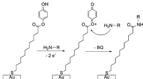
**Figure 1.** Electrochemically induced amide bond formation on a HQ monoester-terminated SAM.
