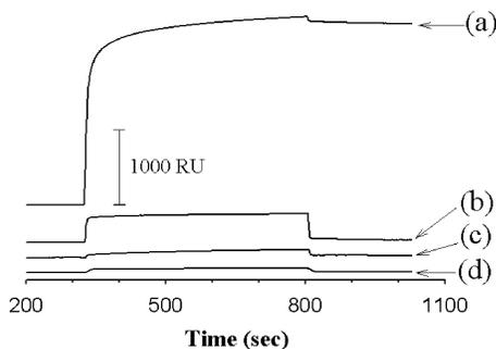
**Figure 3.** SPR sensorgrams of SAM I surfaces treated by various methods. Interaction between (a) SA and the SAM I surface after electrochemical reaction with 1 mM BPA, (b) SA presaturated with excess free biotin and the BPA-reacted surface, (c) SA and the SAM I surface dipped into the same BPA solution at open circuit potential for 45 min, and (d) SA and a freshly prepared SAM I surface.
