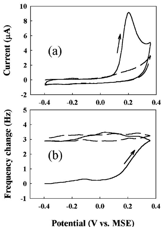
**Figure 2.** (a) Cyclic voltammogram and (b) frequency-potential curve of a **1**-modified quartz crystal (AT-cut 6 MHz; sensitivity, 4.2 ng/Hz) gold electrode in 0.1 M phosphate buffer (pH 7.2) at a scan rate of 50 mV s<sup>-1</sup>. The solid line is the first scan, and the dashed line is the second scan.
