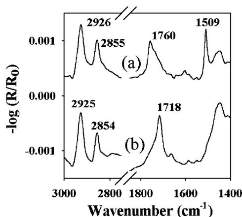
**Figure 3.** Grazing angle FTIR spectra obtained for (a) a freshly prepared **2** SAM and (b) the SAM after electrochemical deprotection.
