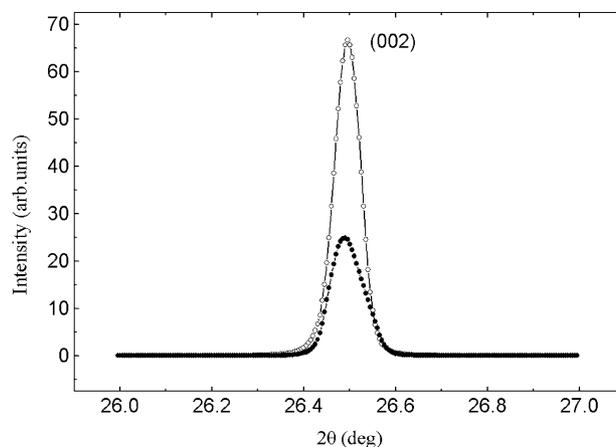
Fig. 2. XRD pattern of HOPG (open circle) and B-doped HOPG (closed circle).
