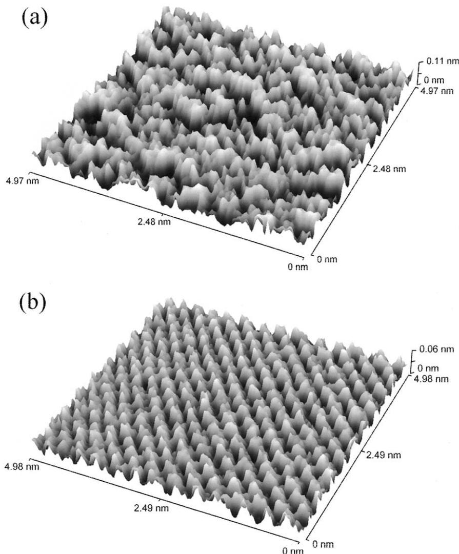
Fig. 4. AFM topographic image obtained from (a) the B-doped HOPG and (b) pure HOPG. The scan rate is 134 Hz with the force constant, 0.032 N/m.
