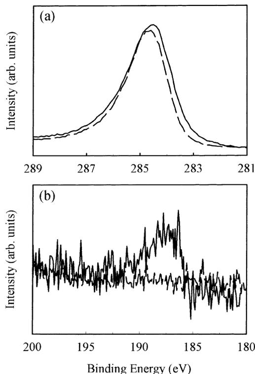
Fig. 1. (a) XPS C 1s spectra and (b) B 1s spectra of HOPG (dashed line) and B-doped HOPG (solid line).
