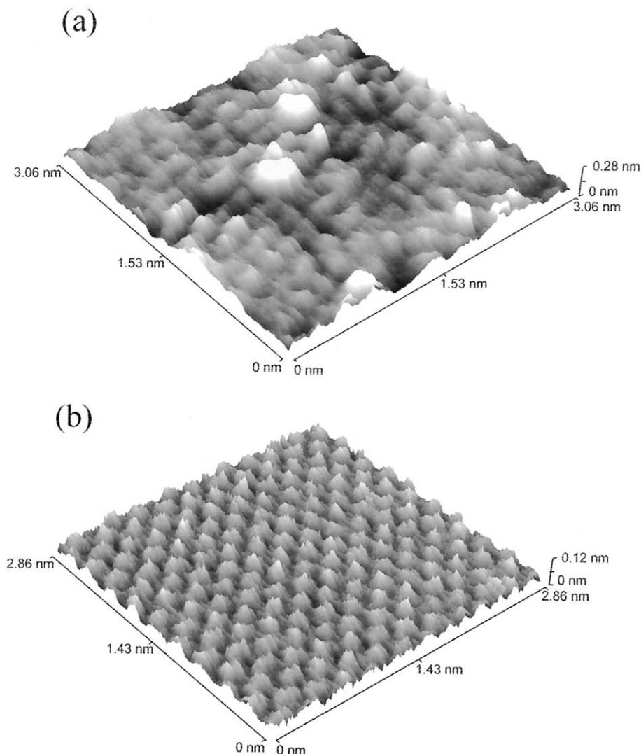
Fig. 3. STM topographic image of (a) B-doped HOPG and (b) pure HOPG. Constant current mode with a scan rate of 30 Hz, sample bias of 100 mV, and tunneling current of 2 nA.
