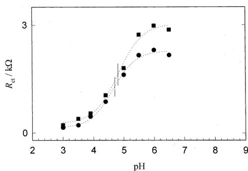
Fig. 7. Faradaic impedance titration curves for pure MPA (●) and 9:1 (MPA + EtSH) mixed (■) SAM. Ionic strength is 0.5 M and coating time is 60 h.
