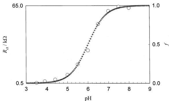
Fig. 4. Experimental plots (O) by faradaic impedance titration for pure MPA SAM and calculated plots (+) based on Eq. (2).
