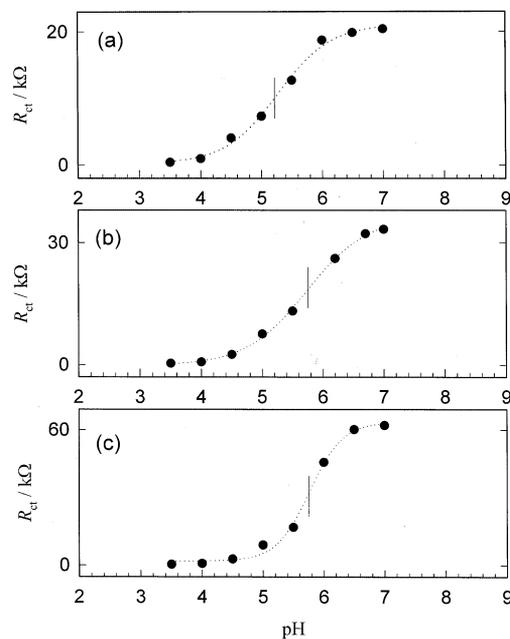
Fig. 5. Faradaic impedance titration curves for: (a) pure MPA; (b) 9:1 (MPA + EtSH) mixed; and (c) 1:1 (MPA + EtSH) mixed SAM. Ionic strength is 0.1 M and coating time is 1 h.
