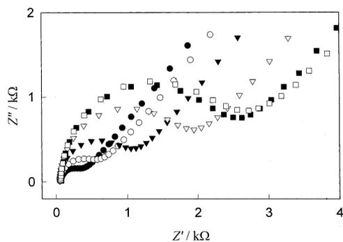
Fig. 6. Complex impedance plots of a MPA modified electrode in the presence of 0.5 mM  $\text{Fe}(\text{CN})_6^{3-}$  at pH 3.5 (●), 4.0 (○), 4.5 (▼), 5.0 (▽), 5.5 (■), and 6.0 (□) solutions of 0.5 M ionic strength. Coating time is 60 h.
