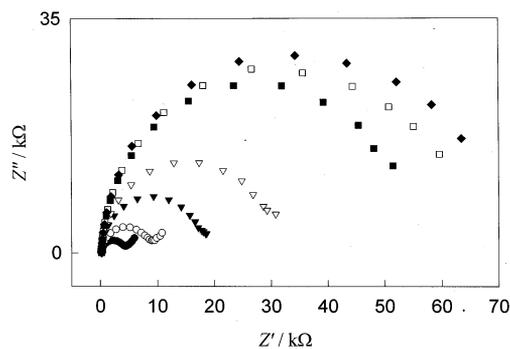
Fig. 2. Complex impedance plots of a MPA modified electrode in the presence of 0.5 mM  $\text{Fe}(\text{CN})_6^{3-}$  at pH 4.5 (●), 5.0 (○), 5.5 (▼), 6.0 (▽), 6.5 (■), 7.0 (□), and 7.5 (◆) solutions of 0.1 M ionic strength. Coating time is 60 h.
