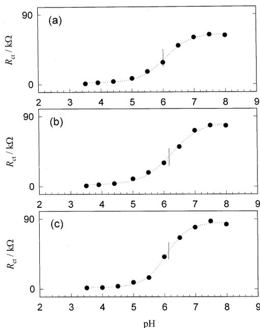
Fig. 3. Faradaic impedance titration curves for: (a) pure MPA; (b) 9:1 (MPA + EtSH) mixed; and (c) 1:1 (MPA + EtSH) mixed SAM. Ionic strength is 0.1 M and coating time is 60 h.
