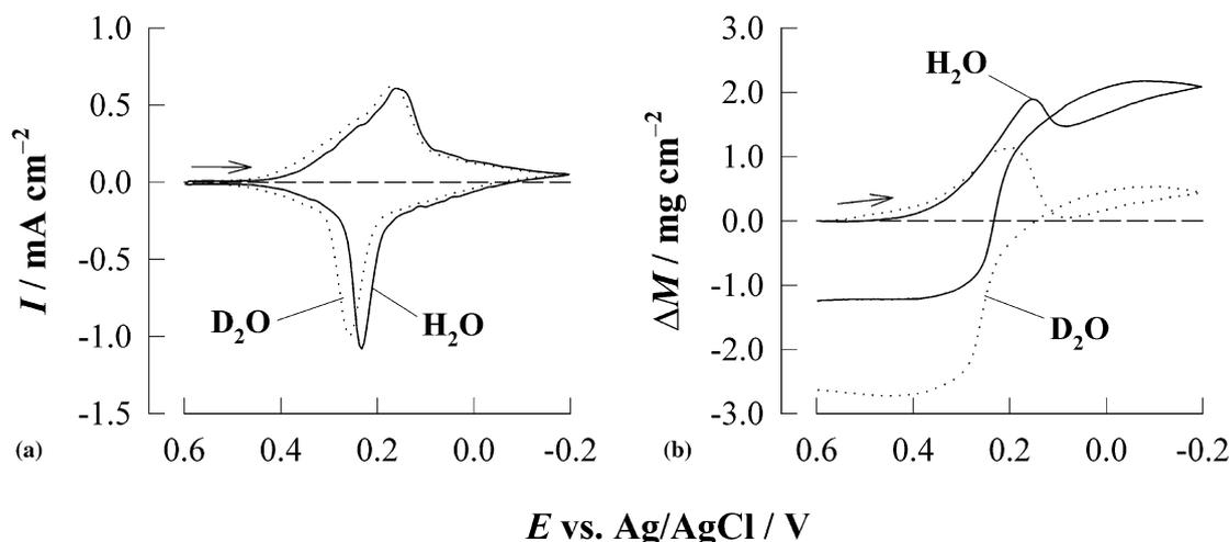
Fig. 4. (a) Cyclic voltammogram and (b) mass change diagram of PB in 0.5 M  $\text{KNO}_3/\text{H}_2\text{O}$  (solid line) and  $\text{KNO}_3/\text{D}_2\text{O}$  (dotted line) ( $Q_{\text{d}} = 10 \text{ mC/cm}^2$ , scan rate = 10 mV/s).
