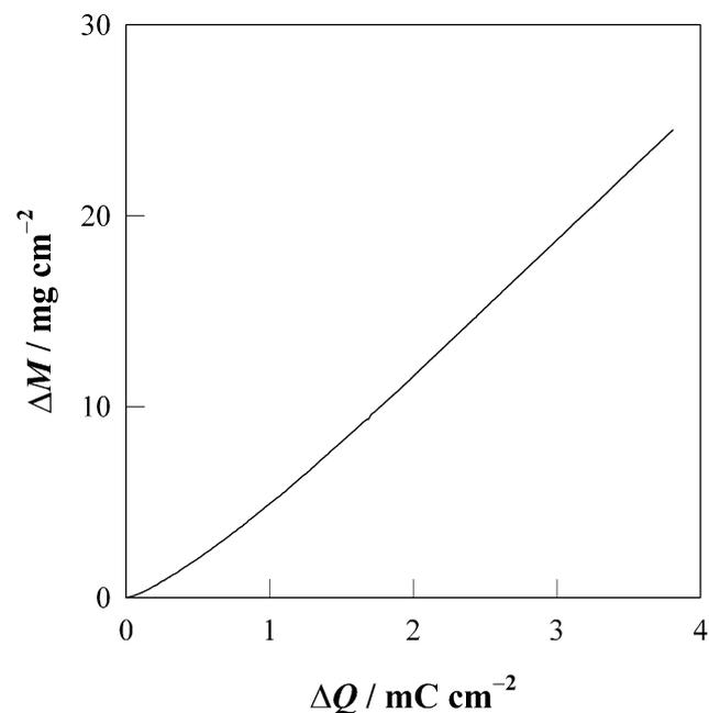
Fig. 1. Mass change ( $\Delta M$ ) vs charge change ( $\Delta Q$ ) diagram during the potentiostatic electrocrystallization of PB at  $E = 0.6 \text{ V}$  on gold electrode in the acidic solution containing  $\text{Fe}^{3+} + \text{Fe}(\text{CN})_6^{3-}$ .
