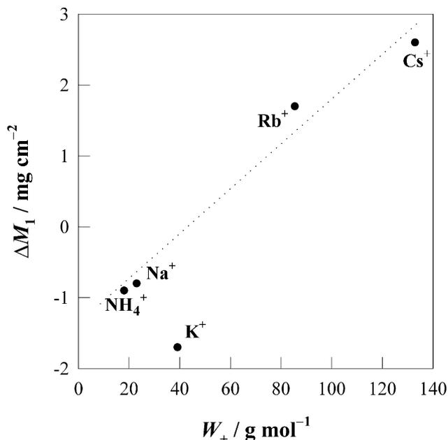
Fig. 3. Irreversible mass change ( $M_1$ ) vs molar mass of cation ( $W_+$ ) diagram of PB after the first scan in 0.5 M solutions of  $\text{NO}_3^-$  ( $\text{Cl}^-$  for  $\text{NH}_4^+$ ) and various kinds of cations ( $Q_{\text{dep}} = 10 \text{ mC/cm}^2$ , scan rate = 10 mV/s).
