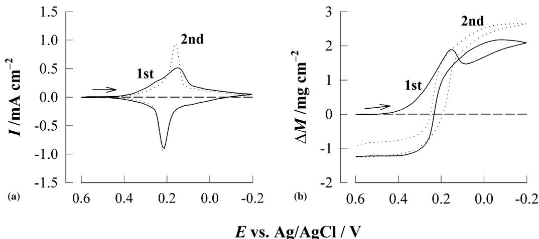
Fig. 2. (a) Cyclic voltammogram and (b) mass change diagram during the first two cyclic scans of PB in 0.5 M KNO<sub>3</sub> ( $Q_{\text{dep}} = 10$  mC/cm<sup>2</sup>, scan rate = 10 mV/s).
