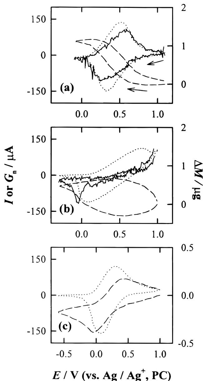
**Figure 3.** (a) Cyclic voltammograms ( $I$  vs.  $E$ ;  $\cdots$ ), normalized mass change rate diagrams ( $G_n$  vs.  $E$ ;  $\text{---}$ ), and mass change diagrams ( $\Delta M$  vs.  $E$ ;  $-\cdot-\cdot-$ ) for a PB film in (a)  $\text{NaClO}_4/\text{PC}$ , (b)  $\text{NaBPh}_4/\text{PC}$ , and (c)  $\text{LiClO}_4/\text{PC}$ .
