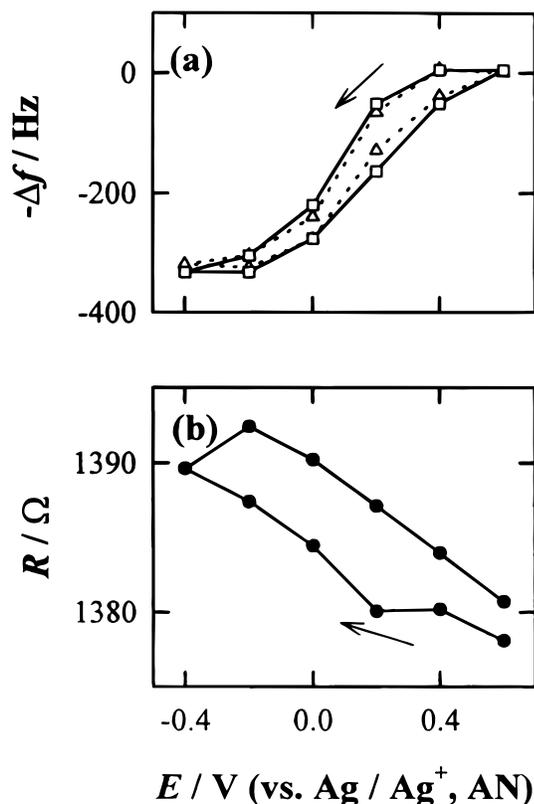
**Figure 1.** (a)  $f_r$  (—□—),  $f_o$  (···△···) changes and (b)  $R_t$  change for a PB film in 1 M NaClO<sub>4</sub>/AN during the electromechanical impedance experiment.
