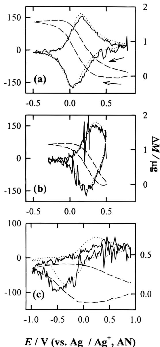
**Figure 2.** Cyclic voltammograms ( $I$  vs.  $E$ ; ···), normalized mass change rate diagrams ( $G_n$  vs.  $E$ ; —), and mass change diagrams ( $\Delta M$  vs.  $E$ ; ---) for a PB film in (a) NaClO<sub>4</sub>/AN, (b) NaBPh<sub>4</sub>/AN, and (c) LiClO<sub>4</sub>/AN.
